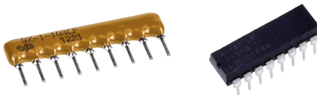
Figure 2.3 Resistor networks come in SIL (left) and DIL (right) packages.
