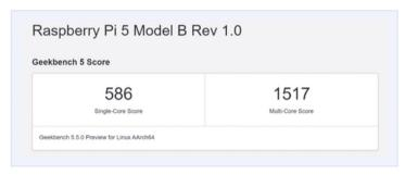
Figure 1.4 Geekbench 5 benchmark scores for the Raspberry Pi 5 (Geekbench)
