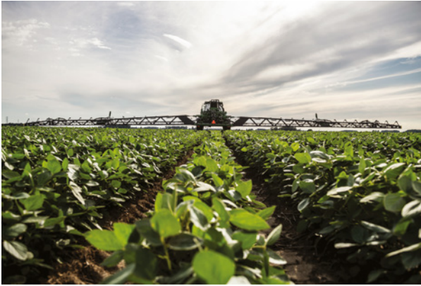
Figure 2.1 An example of Deere's use of advanced innovations that help farmers do more with less is its See & Spray™ technology. The technology enables farmers to only spray herbicides on the weeds, which reduces the amount needed by up to 66%. The technology can "recognize the difference between plants even in conditions that would challenge the human eye. See & Spray has 36 cameras . . . [that] scan more than 2,200 square feet of land and capture 1.2 billion pixels per second. If you tried to match that level of sensing and processing with human eyes, it would take nearly 6,000 people." 4
