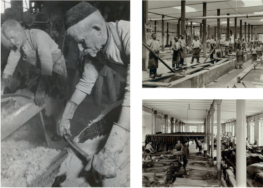
Fig. 6-8 Depilating the skins, 1938 ■ Tanning pits in the tannery in Müllheimer Tal, 1899 ■ Finishing colored skins, 1899
