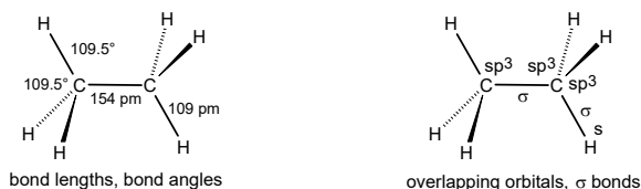
Fig. 4.2. Bond lengths (nuclear distances), bond angles and \sigma bonds of ethane
