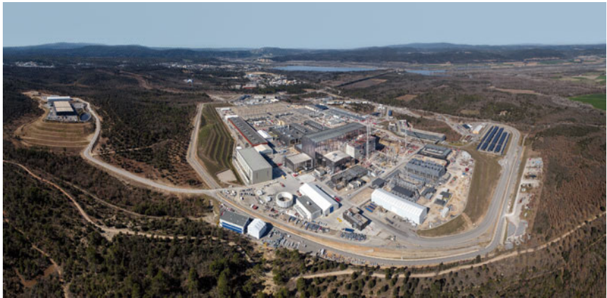
Fig. 1 Aerial view of the ITER worksite in Cadarache (close to Marseille) in March 2023. The site has a total area of 181 ha. (Left) The main warehouse that is used for the storage of the reactor parts delivered by the seven ITER members. (Top right) The headquarters of the international organisation (the building which is bent and has a dark façade). The reactor will be located in the tallest building on the platform that is surrounded by four cranes (beside what is known as the “assembly hall”). Nearly, 5000 people are currently working on the site. From ITER Organization
