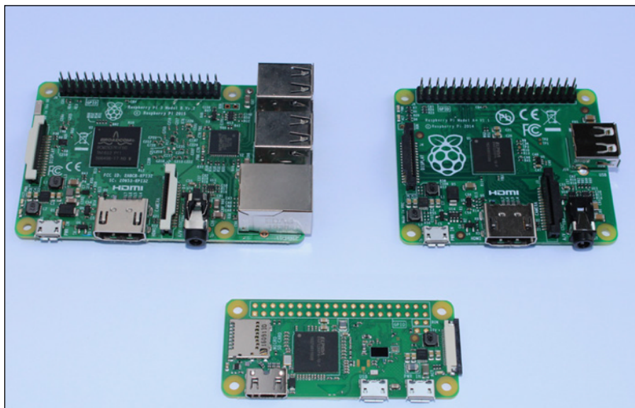
FIGURE 1-2: The Raspberry Pi 3 Model B (top left), Model A+ (top right), and Pi Zero W (bottom).
