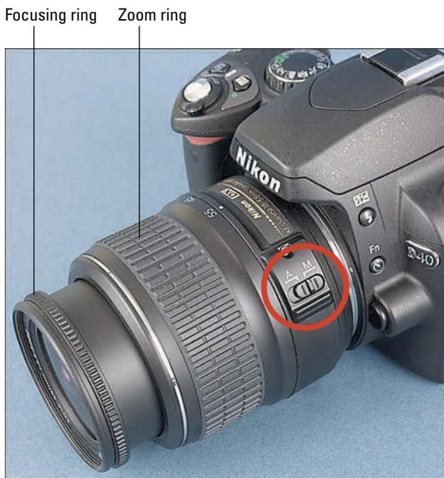
**Figure 1-3:** Set the focusing mode switch to M before turning the manual focus ring.
