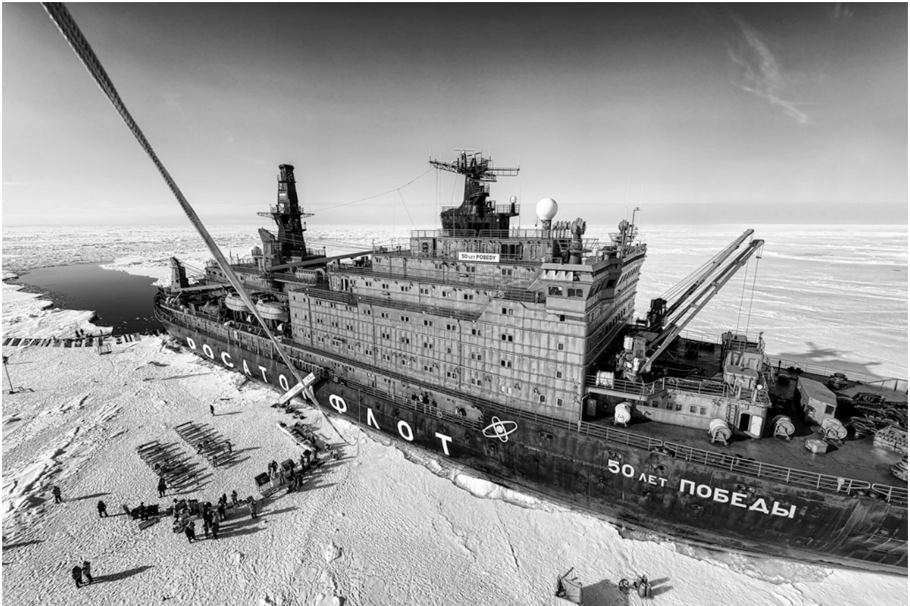
Fig. 4 To reach the North Pole with a surface ship requires something like this Russian vessel, a nuclear-powered icebreaker called the ‘50 Years of Victory’. The ship can break through ice up to 2.8 m thick,
