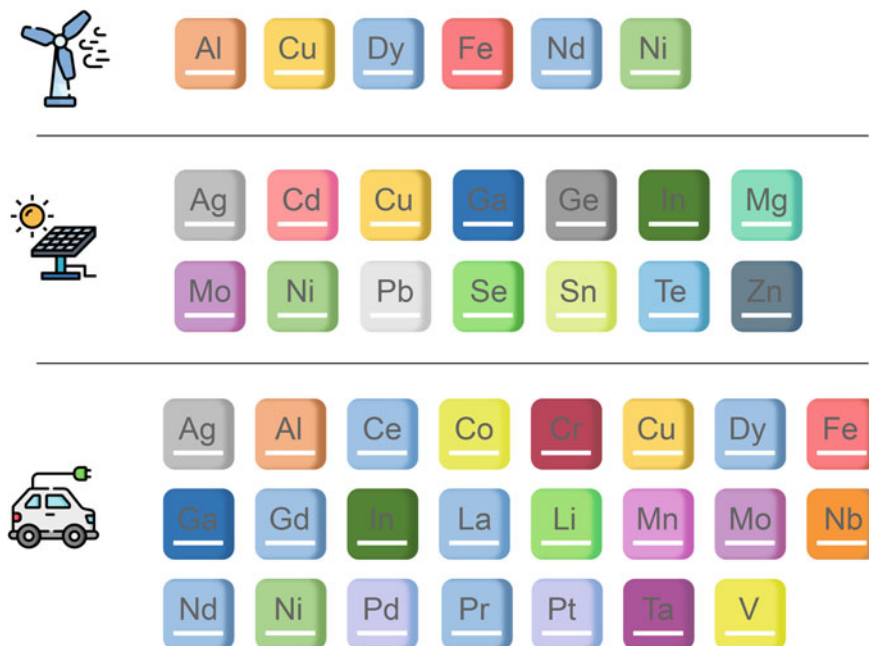
Fig. 1.3 Some of the elements that are used to manufacture clean technologies (Valero et al., 2018)
