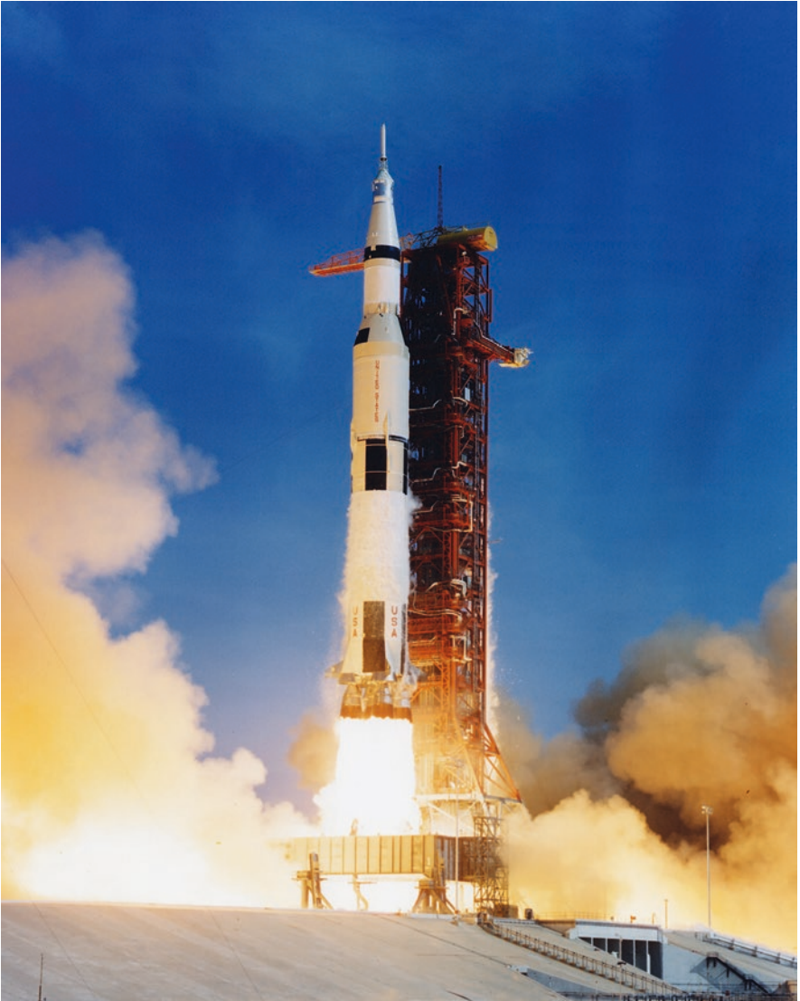
Fig. 1 The Saturn V Moon rocket with Apollo 11 on its way to the Moon. This rocket, the most powerful machine ever built, had a weight of almost 3000 metric tons, a total height of 111 meters, and developed a thrust of 3500 tons, or 160 million horse power. Photo: NASA. No.: AP11-KSC-69PC-442
