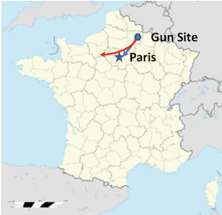
FIG. 1.3 The 1918 “Paris gun”. Shells were fired at Paris from 120 km to the north-east of the capital. Shells curved to the west of the city as a result of the Coriolis Effect ( red arrow ). The gunners soon corrected for this and repeatedly shelled Paris. French map courtesy of Wikipedia Commons
