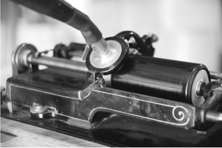
Figure 1.1 Closeup of early Edison cylinder phonograph showing diaphragm and needle, from Paul Bourbin collection.
