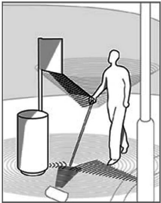
Figure 1.4 The Ultracane mobility aid: ultrasound transducers convert echoes from objects to vibrations in ‘tactors’ in contact with the fingers of the hand holding the cane. This, in turn, enables the brain to build a spatial map of the immediate surroundings (Figure courtesy of Professor Brian Hoyle, University of Leeds.*)
