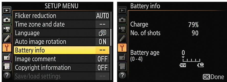
**Figure 1-8:** The Battery Info option on the Setup menu provides details about battery life.
