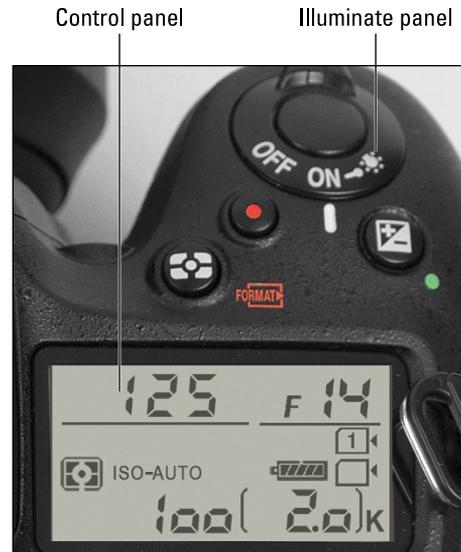
**Figure 1-15:** Rotate the On/Off switch to the light bulb position to illuminate the Control panel.
