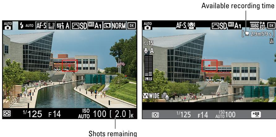
**Figure 1-7:** In Live View mode, the displays offer these hints about memory-card capacity.
