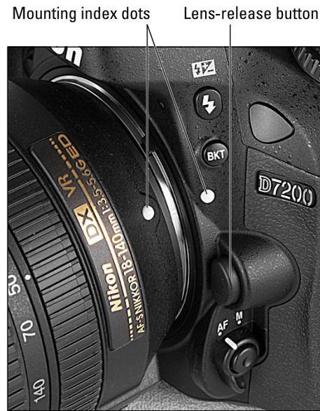
**Figure 1-1:** Align the white dot on the lens with the one on the camera body.
