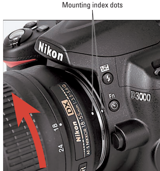
Figure 1-1: When attaching the lens, align the index markers as shown here.
