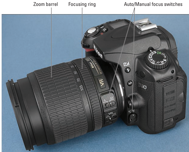
Figure 1-3: On the 18–105 kit lens, the manual-focusing ring is set near the back of the lens, as shown here.
