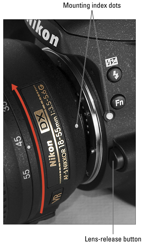
Figure 1-1: When attaching the lens, align the index markers as shown here.
