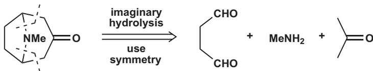
This was a famous synthesis because it is so short and simple and also because it makes a natural product in a way that imitates nature. The reaction is carried out at pH 7 in water. In fact Robinson didn't use acetone, as suggested by his 'imaginary hydrolysis', but acetone dicarboxylic acid. This procedure is an improved one invented by Schöpf<sup>2</sup> in 1935.
