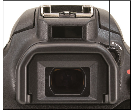
FIGURE 1-5: Use this dial to adjust the viewfinder focus to your eyesight.
