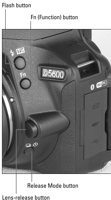
FIGURE 1-8: Press the Flash button to use the built-in flash in P, S, A, or M mode.
