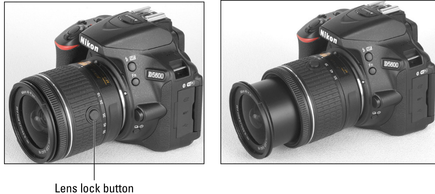
FIGURE 1-5: If using a retractable lens, press the lens lock button while rotating the lens barrel to extend and retract the lens.
