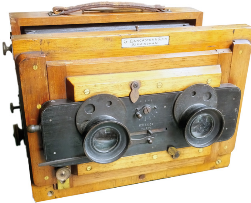
Bild 2.8 J. Lancaster & Son Stereoscopic Camera 1898 (Quelle: https://commons.wikimedia.org/wiki/Category:Stereo_cameras , Creative Commons, Fotograf: Clem Rutter)
