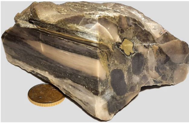
Fig. 1.16 In this strongly deformed conglomerate, the shape of the pebbles is still recognisable on the right cut surface, but in the other spatial direction they have been extremely elongated. Sample from Bygdin, Norway (© Florian Neukirchen 2009)
