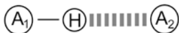
Fig. 1.4 Diagram of a hydrogen bond. The hydrogen atom forms a covalent bond with atom A_1 and a hydrogen bond with atom A_2 . Atoms A_1 and A_2 can be either nitrogen or oxygen atoms
