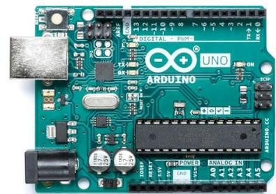
Abb. E-8 Arduino Uno (Rev. 3)
