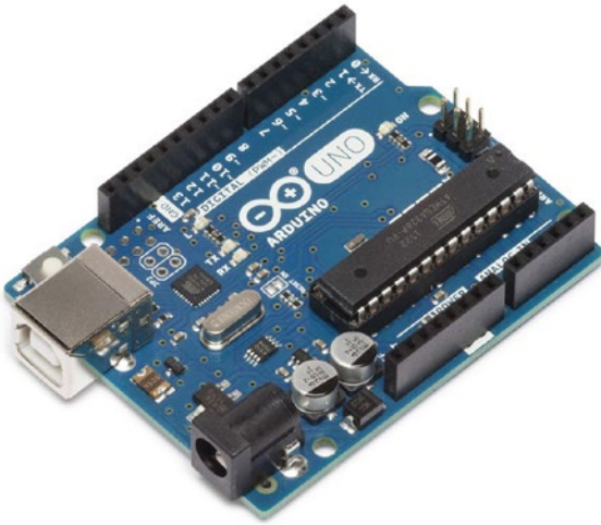
Figure 1-2. Arduino UNO Rev3 board. Image courtesy of arduino.cc
