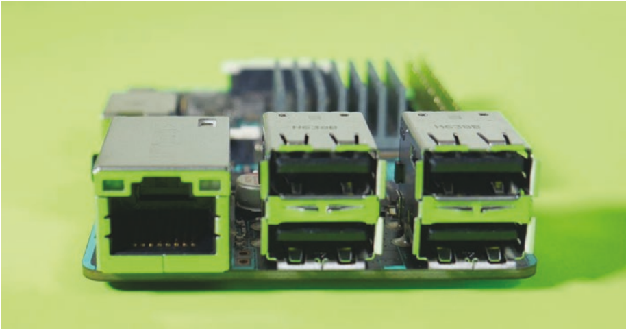
Figure 1-2. The Tinker Board's four USB 2.0 ports and Ethernet port
