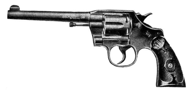
Fig. 2.—COLT ARMY SPECIAL REVOLVER Six shots; 6 inch barrel; weight, 2 lbs. 3 oz., .38 cal.
