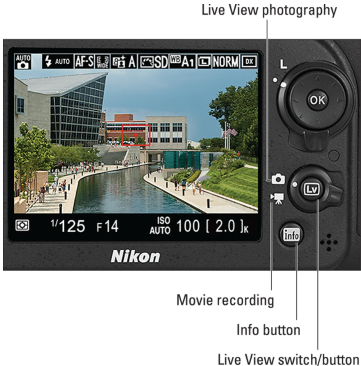
**Figure 1-4:** Press the LV button to toggle Live View on and off.
