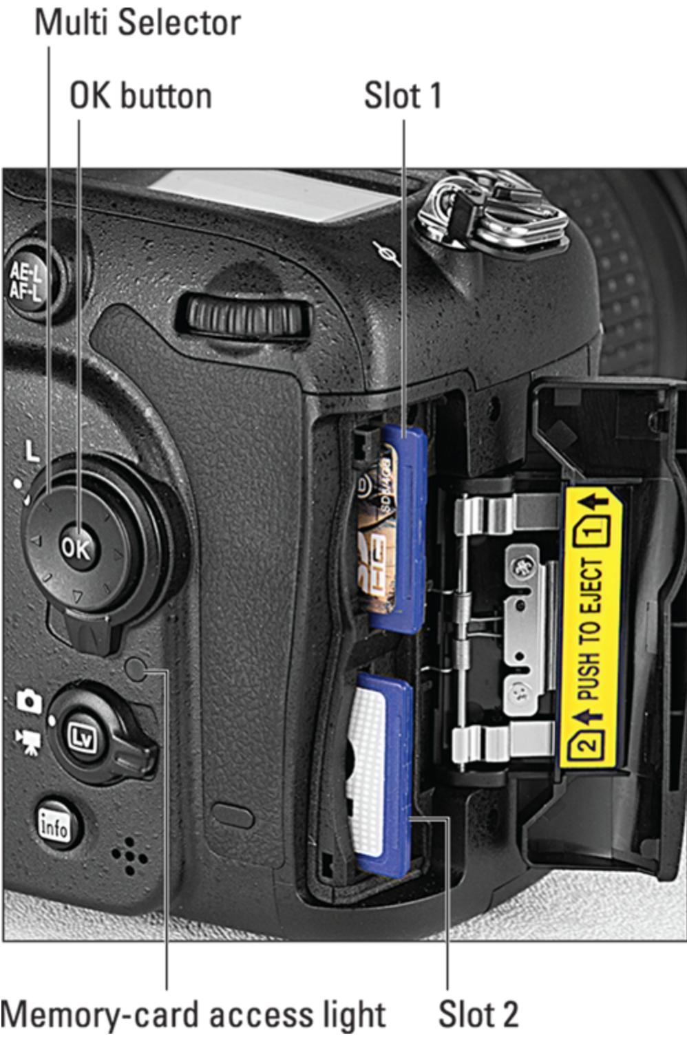
**Figure 1-2:** You can install one or two SD memory cards.
