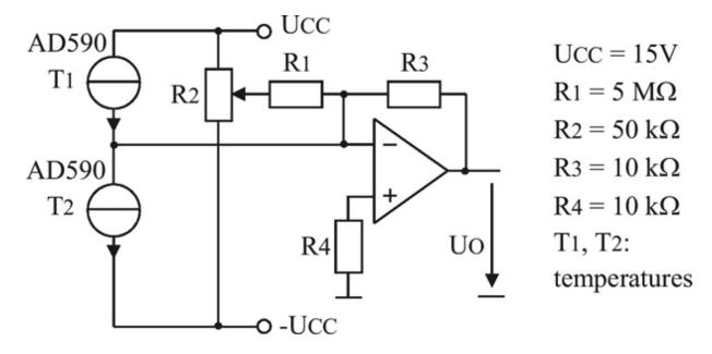
The AD590 is a temperature sensor, which provides an impressed current of  $1\mu A/K$ .
