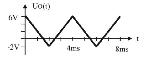
Develop a circuit which generates the above waveform. There are rail to rail Operational Amplifiers available with a supply voltage of +/-15V. Resistors may be used any desired, capacitors from the standard series E6. It is important to ensure that no OpAmp output is loaded with less than  $2k\Omega$ .
