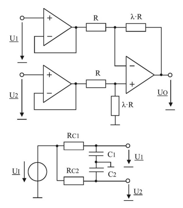
The inputs of the circuit are supplied with wires of different length. These are modelled by RC elements. Both lines are connected together on the other side. There, the voltage Ui is applied.
