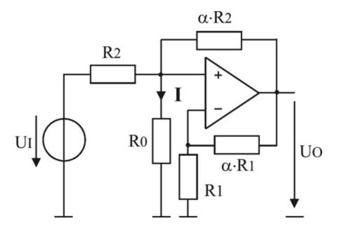
It is assumed that the operational amplifier will operate in negative feedback.
