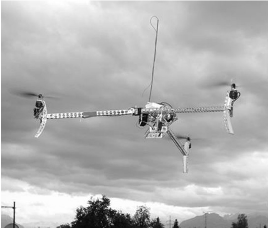
Figure 1: Tricopter with aluminum frame, photo: Karl-Heinz Wolf.
