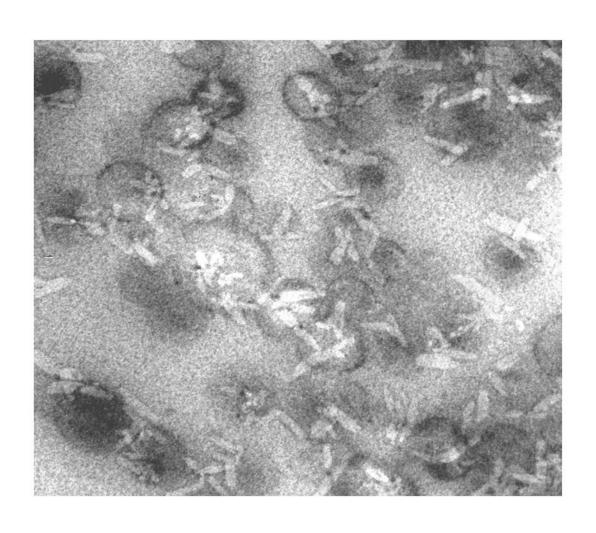
Cover picture: SEM picture of a rubber phase in polystyrene
