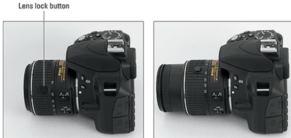
Figure 1-3: Press the lens lock button while rotating the lens barrel to extend and retract the lens.
