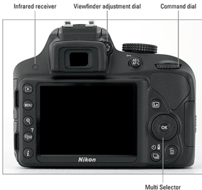
Figure 1-6: Use the Multi Selector to navigate menus and access certain other camera options.
