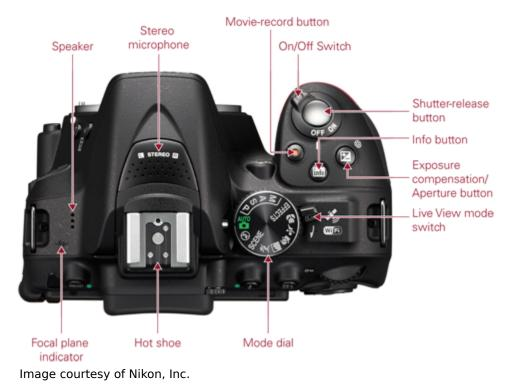
**1.1** The controls on top of the camera.
