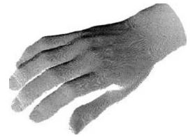
**3D data acquisition**: Sampling data in all three spatial dimensions. There is a variety of ways to perform this sampling, e.g., using <u>structured light triangulation</u>. [FP03:21.1]
