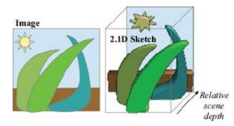
**2.5D image**: A <u>range image</u> obtained by scanning from a single <u>viewpoint</u>. It allows the data to be represented in a single image array, where each pixel value encodes the distance to the observed scene. The reason this is not called a <u>3D image</u> is to make explicit the fact that the back sides of the scene objects are not represented. [SQ04:4.1.1]
