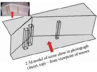
**2.5D sketch**: Central structure of <u>Marr's Theory</u> of vision. An intermediate description of a scene indicating the visible surfaces and their arrangement with respect to the viewer. It is built from several different elements: the contour, texture and shading information coming from the <u>primal sketch</u>, stereo information and motion. The description is theorized to be a kind of buffer where
