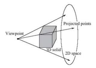
For example, the main steps for a computer graphics projection are as follows: apply normalizing transform to 3D point world coordinates; clip against canonical view volume; project onto projection plane; transform into viewport in 2D device coordinates for display. Commonly used projection functions are <u>parallel projection</u> and <u>perspective projection</u>. [JKS95:1.4]
