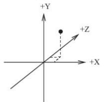
**3D data**: Data described in all three spatial dimensions. See also <u>range data</u>, <u>CAT</u> and <u>NMR</u>. [WP: <u>3D data acquisition and object reconstruction</u>] An example of a 3D data set is:
