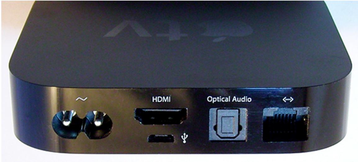
**1.6** The back of the Apple TV features an Ethernet port, an optical digital audio port, an HDMI port, a micro USB port, and a power connector.
