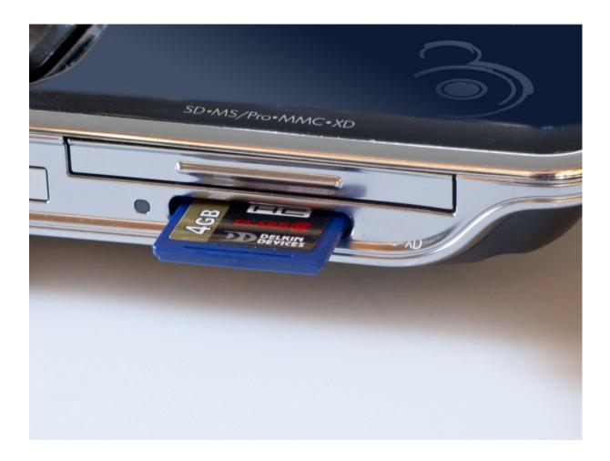
A memory card is a small, removable digital storage device used in many electronic gadgets such as digital cameras, MP3 players and so on. Many laptops feature memory card readers – small slots into which you can insert a memory card. You can then view the contents of the memory card and even use the memory card as an external storage device to save data from your laptop.
