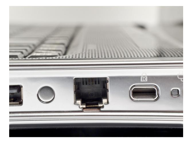
Although most people use an Ethernet cable or a wireless signal to access the Internet, there may be times when you must use a phone line. If you need to use a phone line to dial up your Internet connection, you can plug a phone cable into the modem jack to pick up a signal.
