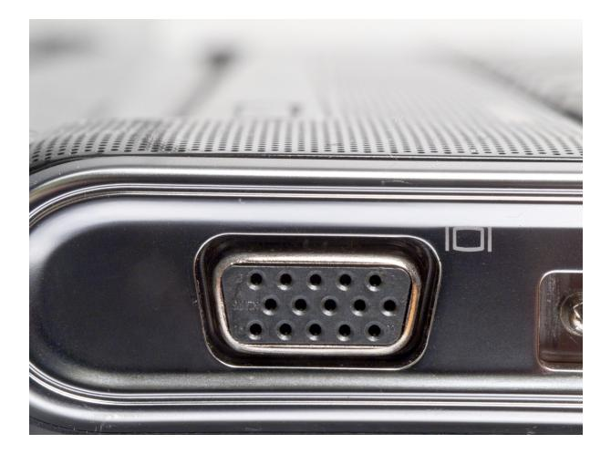
Some laptop computers include a monitor port. If you want to connect an external monitor to your laptop – for example, to show a presentation on a larger screen or if you use a dual-monitor system in your workflow – you can connect a standard monitor cable to the laptop's monitor port.
