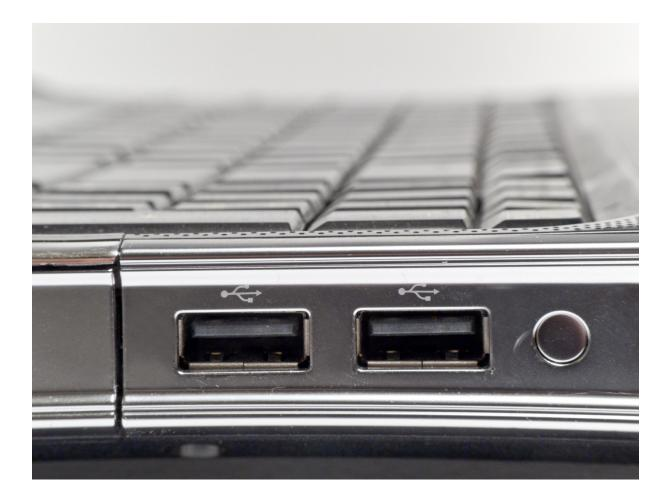
You can use a universal serial bus (USB) port to connect a wide variety of devices, from a flash drive for data storage to a printer or digital camera. Devices that can be connected via USB are generally plug-and-play – that is, you need not restart your computer to use them after connecting them via a USB cable. Windows can automatically install many USB devices when you connect them, requiring no additional input from you.
