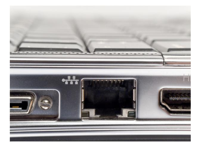
You use an Ethernet jack to connect your computer to a router that controls your local area network (LAN) through a coaxial or fibre-optic cable. You can also use an Ethernet jack to establish a high-speed connection to the Internet. You simply plug the Ethernet cable into the Ethernet jack on your laptop and then connect the other end of the cable to a high-speed modem.
