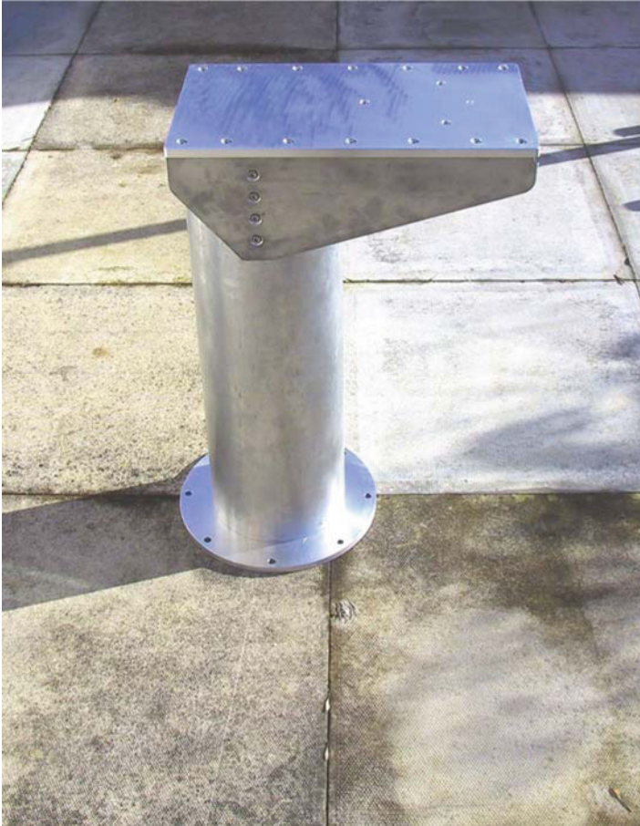
Figure 1.3 The custom-made all-aluminium Equatorial mode pillar.
