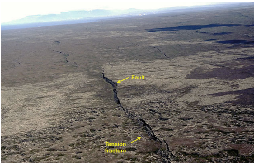
Fig. 2.5 Aerial view of fractures formed by plate-tectonic forces in pahoehoe (smooth-surface) basaltic lava flows of the Reykjanes Peninsula. View (facing or looking) northeast towards the capital region and the mountain Esja. The long fractures are normal faults, the shorter ones tension fractures (their formation is discussed in Chap. 5). The longest fractures reach lengths of many kilometres. These fractures, and those seen in Fig. 2.6, belong to the northwestern part of the Reykjanes Volcanic System (Fig. 2.3); more specifically to the so-called Vogar Fissure Swarm of that system—Vogar is a village close to the second stop in Fig. 2.1. Most of the lava seen here belongs to Thrainsskjöldur, but the closest lava flow, where the main fault in the centre is ending, is the margin of the Arnarseturshraun lava flow
