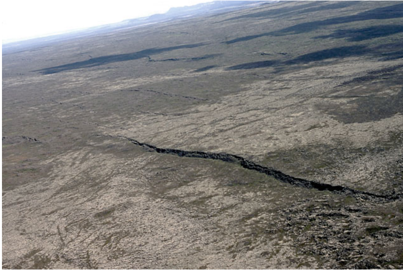
Fig. 2.6 Aerial view of fractures in pahoehoe basaltic lava flows on the Reykjanes Peninsula. View southeast, the main fracture is a normal fault; the lava surface to the left of the fault (closer to you) has subsided by several metres relative to the lava surface to the right of the fault. Several other normal faults are seen here, but also tension fractures. These fractures are part of the Vogar Fissure Swarm of the Reykjanes Volcanic System (Fig. 2.3). See the caption to Fig. 2.5 for more details
