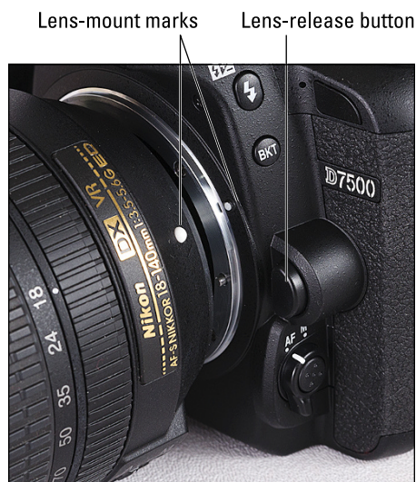
FIGURE 1-1: Align the white dot on the lens with the one on the camera body.
