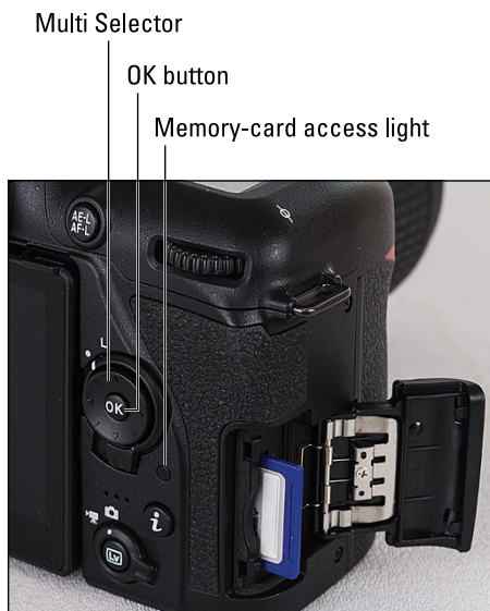
FIGURE 1-2: Insert the memory card with the label facing the back of the camera.
