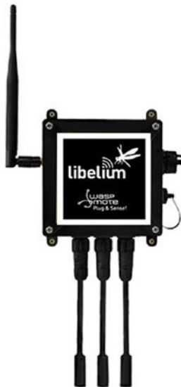
Figure 1-12. Waspote Plug & Sense (courtesy of www.libelium.com )
