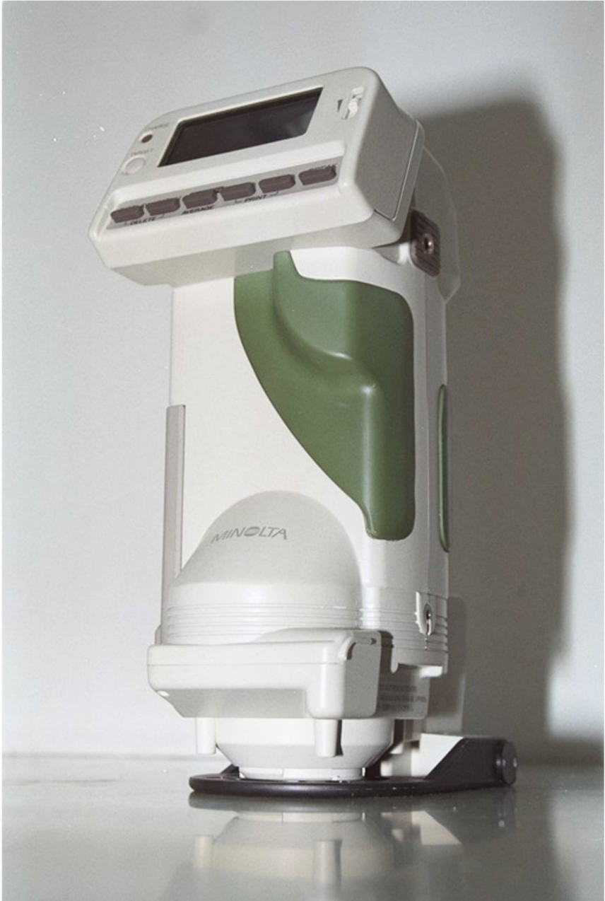
Abb. 3.2-2 Spektralphotometer CM-503c (Minolta, Osaka/Japan).
