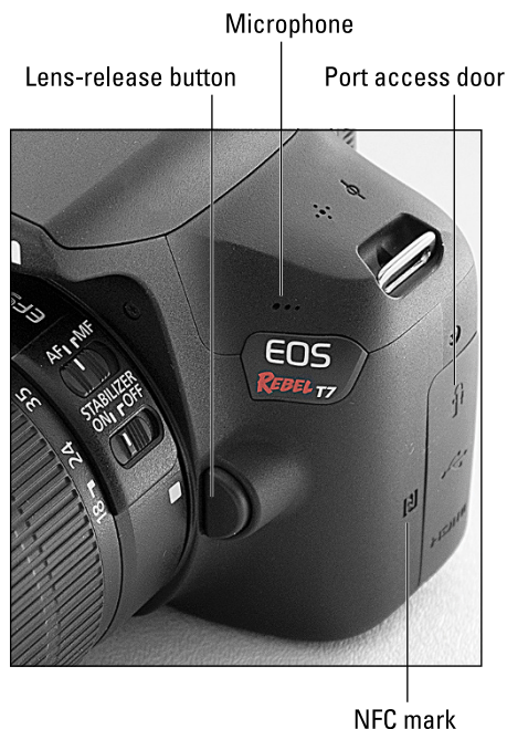
FIGURE 1-6: When recording movies, be careful not to cover the microphone with your finger.
