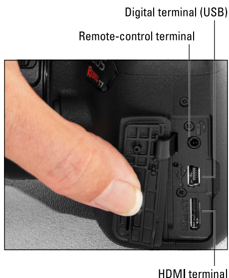
FIGURE 1-7: Inputs for connecting the camera to other devices are found under the cover on the left side of the camera.
