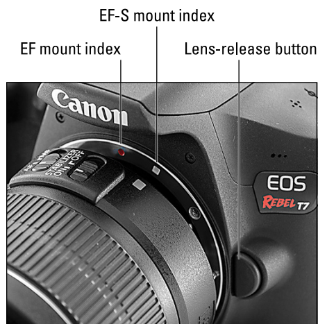
FIGURE 1-1: Align the mounting index on the lens with the one on the camera body.
