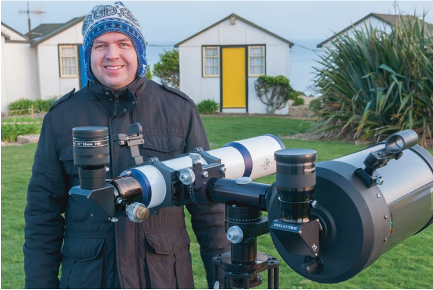
Fig. 2.8 Jonathan Daniels, LAS member who regularly demonstrates star-hopping, with his altazimuth mount supporting a wide field refractor for finding and locating and a larger, long focal length Schmidt Cassegrain telescope for higher power and more detailed views. Note the red dot finders mounted on each. (Image by Andy Gannon)
