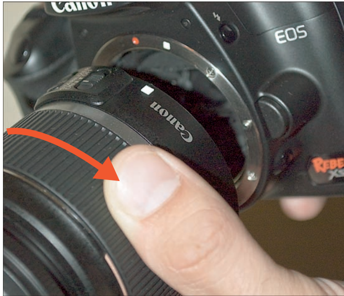
Figure 1-2: Place the lens in the lens mount with the mounting indexes aligned.
