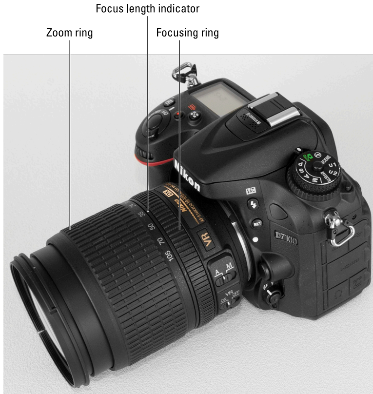
Figure 1-5: On the 18–105mm kit lens, the manual-focusing ring is set near the back of the lens.
