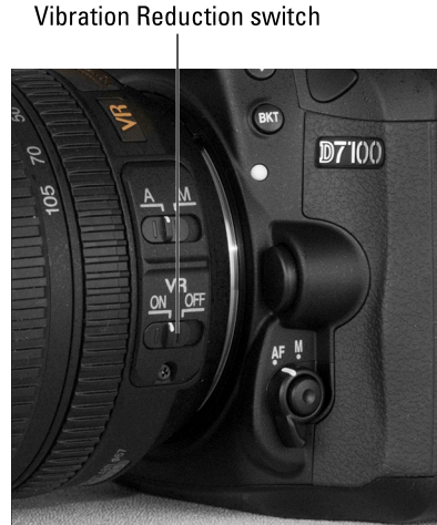
Figure 1-6: Turn on Vibration Reduction for sharper handheld shots, but turn off the feature when you use a tripod.
