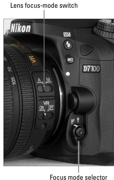
Figure 1-4: Set the focus mode both on the camera body and the lens.
