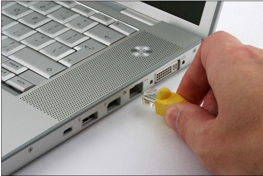
Figure 1-6: An Ethernet port and cable.
