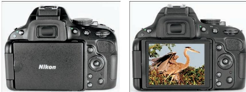
**Figure 1-1:** Here you see just two of the possible monitor positions.
