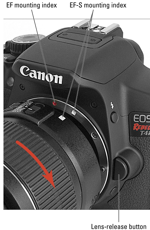
Figure 1-1: Place the lens in the lens mount with the mounting indexes aligned.
