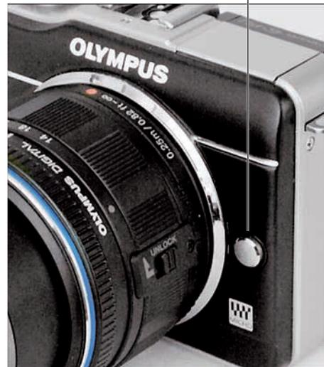
**Figure 1-6:** To disengage the lens, press this button.
